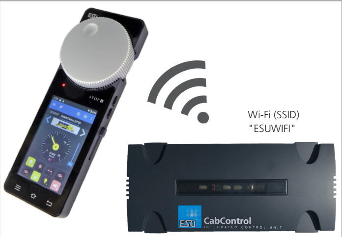
Fig. 14: Island operation with ESU CabControl ICU
